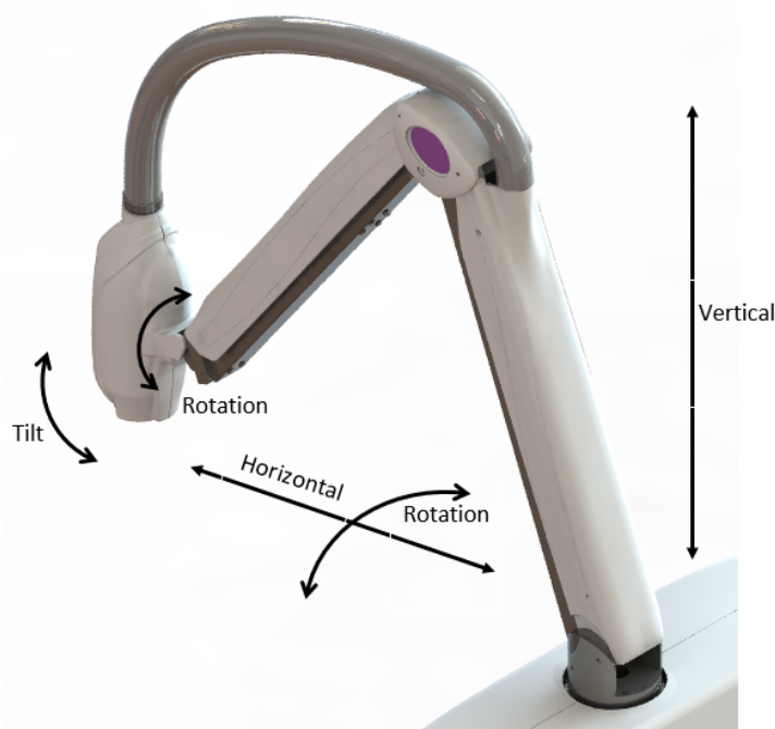
Figure 2-10: Support Arm Range of Movement
