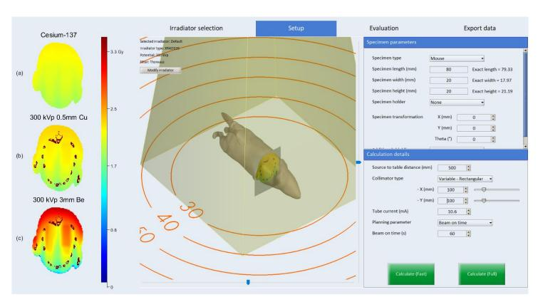
Dose calculations using 3 different radiation sources to deliver 2 Gy mean dose to the liver. Note significant differences in 3D dose distribution between (a) Cs-137, and (b) 300 kV X-rays with hard filter and (c) no filter
